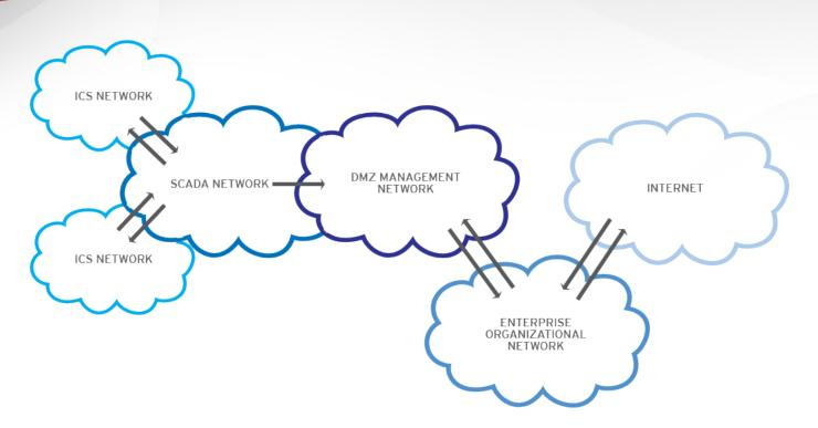
Figure 1. Segmentation: Separation of functionality
