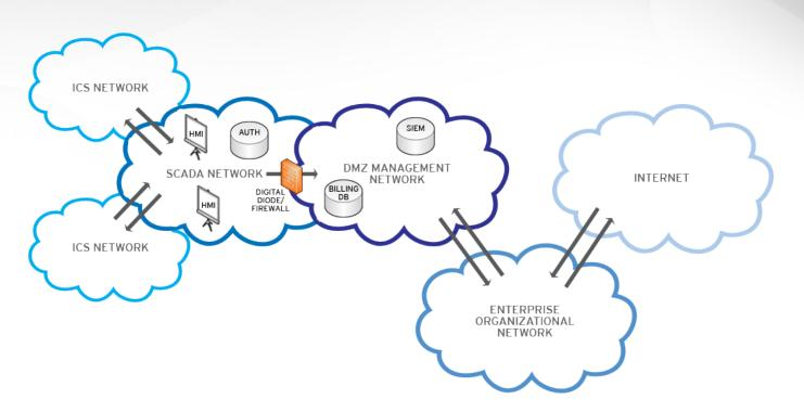
The device that has been added is a specialized firewall, one that only lets traffic flow in one direction, also known as a "digital diode" or a "unidirectional firewall." A digital diode is a specialized device that only allows optical light to propagate in one direction, thus truly only allowing unidirectional traffic flow.
