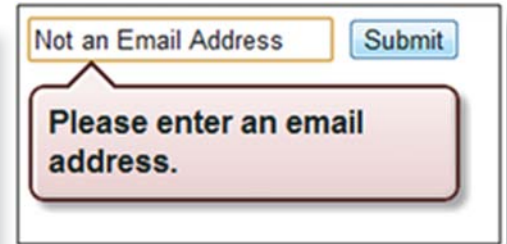
Figure 7. Page that uses the code for the simple form validation with HTML5 in Figure 6
