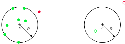
(a) Learning stage: the center c and the radius R of the sphere are determined. (b) Classification stage: new data are accepted (green) or rejected (red).
